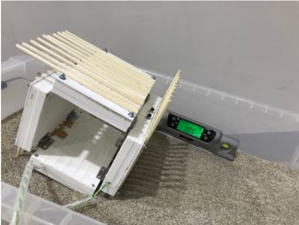
Fig.20 Going up slope of 30 degrees
