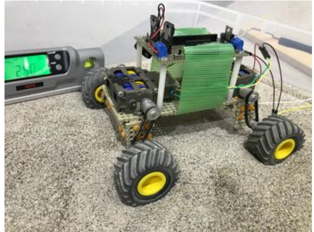
Fig.17 Poor condition of on loose soil : wheel type
