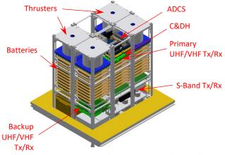
Fig. 4. Core Structure Subsystems (panels not shown)
