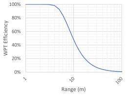
Fig. 8. WPT Range vs. Predicted Efficiency
