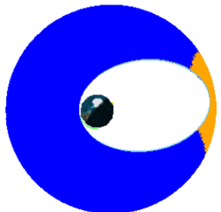
Figure 10. The trajectory for transferring from the GTO to Round orbit ( Orange and blue line indicate maneuver and cruise respectively )
