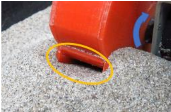
Fig. 16 Situation of excavation using proposed wheel
