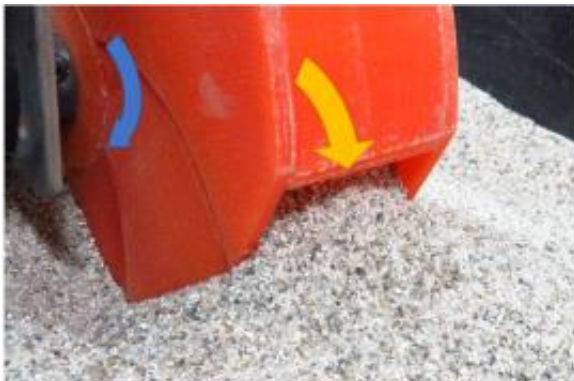
Fig. 17 Situation of ejection using proposed wheel
