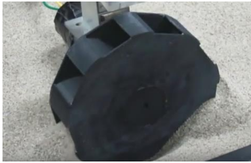
Fig. 15 Situation of excavation using proposed wheel(30sec later)
