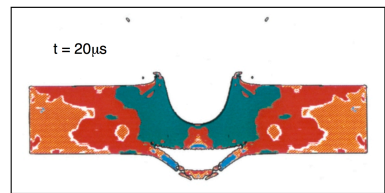
Fig.2 hydrocode simulation of internal failure of rear wall
