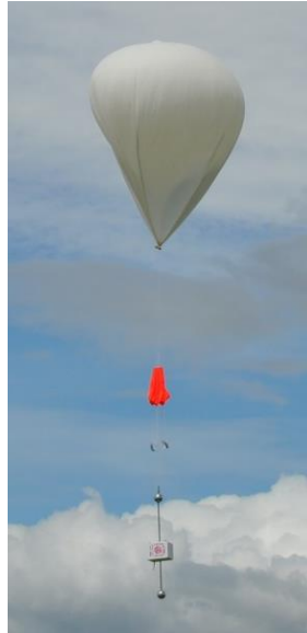
Figure.2.20 One-axis double sphere electric field probe for balloon experiment.
