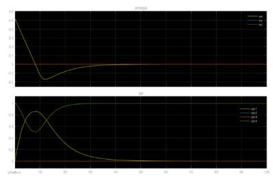
Figure 19: Angular rate (rad/s) and quaternion error over time (s) for detumbling.
