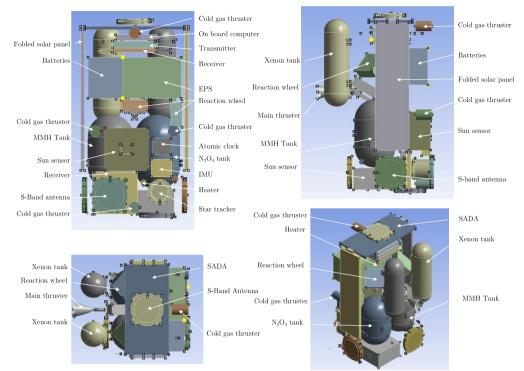
Figure 10: Assembly of the different components inside the spacecraft
