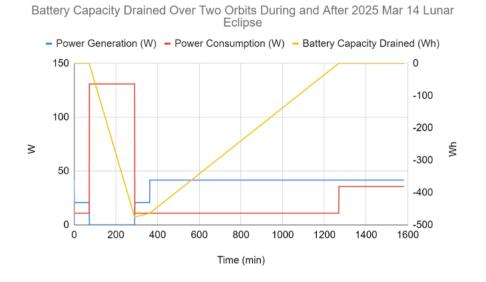
Figure 25: Simulation result for drained battery capacity over two orbits during and after the longest Lunar eclipse. [11]
