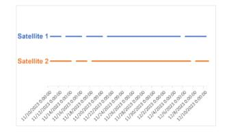
Figure 30: GMAT simulation result for the time when the angular separation of the Earth and the Moon is suitable for simultaneous communication (>30°), for two satellites located 120° apart in the mission orbit, over the first month of the planned mission time.
