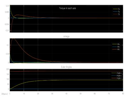
Figure 22: Torque in each axis (Nm), angular velocity (rad/s) and Euler angles (degree) over time (s) for attitude maneuver of 90°.
