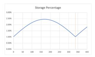
Figure 17: Percentage of maximum momentum storage in use by z-axis reaction wheel over a cycle (until red line).
