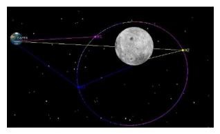
Figure 2: The mission orbit in STK showing LOS with a ground station on the Earth for all three satellites.
