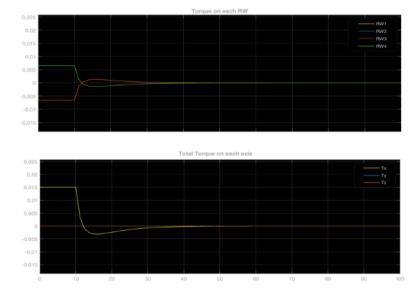
Figure 20: Reaction wheels' torque and total torque (Nm) for detumbling over time (s).
