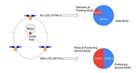
Figure 24: Assumed durations of operational modes over one orbit
