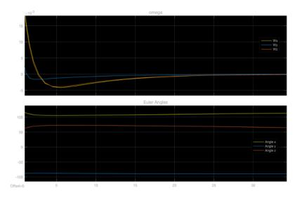
Figure 21 Angular velocity (rad/s) and Euler angles (degrees) over time (s) for attitude maintenance in the presence of disturbances.
