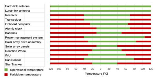
Figure 12: Temperature range of each component
