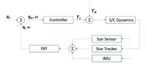
Figure 18: MORSE's ADCS schematic without RCS,  $T_c$ and  $T_d$  represent the control and disturbance torques respectively.
