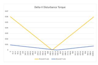
Figure 16: Main thruster disturbance torque (Nm) in 2axis during propulsion mode operation (1040s).
