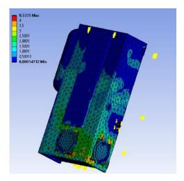
Figure 8: Equivalent Von mises stresses put in the case -6G in axis direction /-5G in orthogonal direction.
