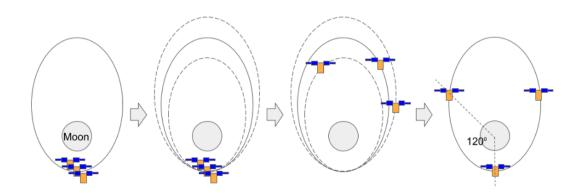
Figure 4: Orbital phasing maneuver
