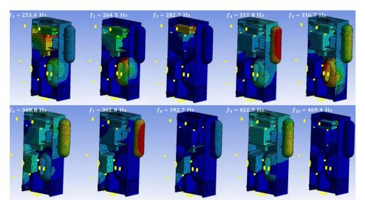
Figure 6: Deformation of the first 10 modes
