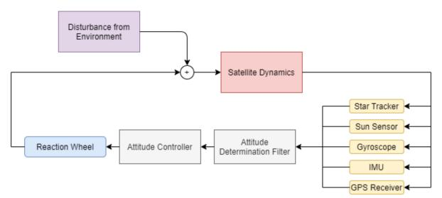
Figure 2.6 The architecture of ADCS in the ALICE satellite
