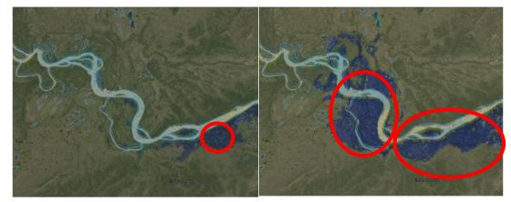
Figure 1.3 Ice-jam floods imagery from the Suomi NPP satellite changed in 12 hours (the red region is flooding water) [3]
