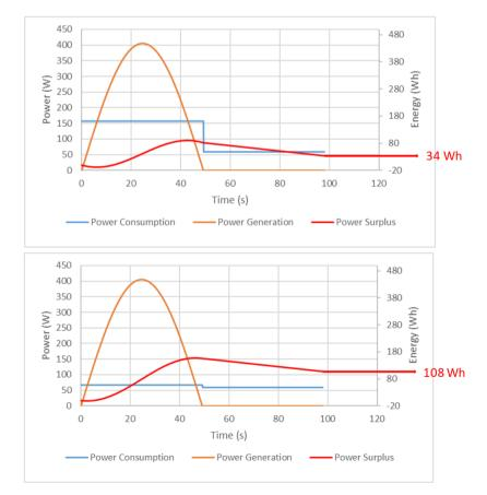
Figure 2.8 Power and energy of mode 1 (top) and 2 (bottom)
