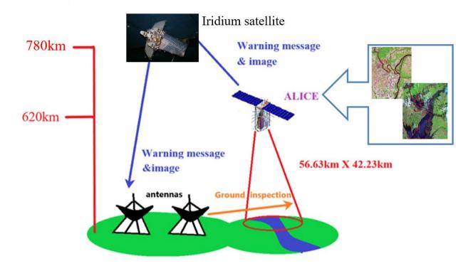
Figure 1.4 The schematic diagram of the ALICE mission
