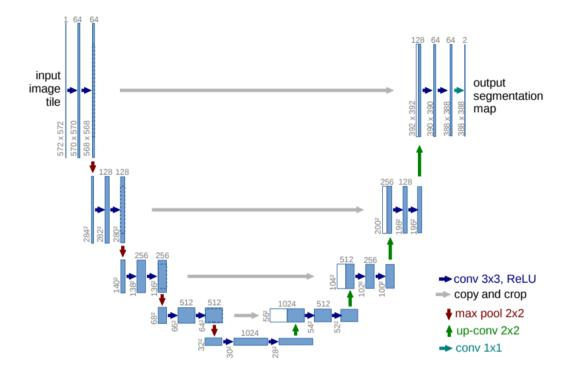
Figure 2.21 U-net architecture (example for 32x32 pixels in the lowest resolution). Each blue box corresponds to a multi-channel feature map. The number of channels is denoted on top of the box. The x-y-size is provided at the lower left edge of the box. White boxes represent copied feature maps. The arrows denote the different operations.
