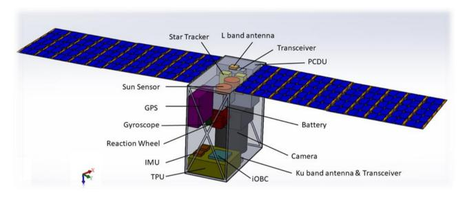
Figure 2.2 The major instruments of the ALICE microsatellite Table 2.3 Mass budget, the mass and volume of each instrument in the ALICE.
