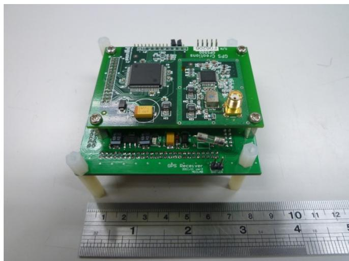
Figure 38. GPSR Payload Prototype
