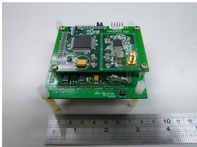
Figure 38. GPSR Payload Prototype
