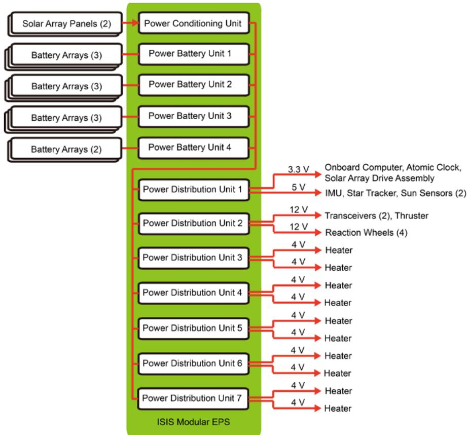
Figure 23: Block diagram of the electrical power system
