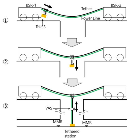
**Fig. 3.** The TrUSS provides tethered (black lines) horizontal and vertical positioning and power (green) for the scientific payloads (VAS+MMRs).
