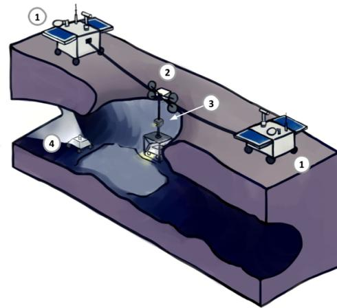
**Fig. 1.** Artistic impression of the ARETHUSA Lunar Platform (LP) exploring a lunar lava tube via its skylight. The LP consists of: ① Base Station Rovers (BSR, Section 3.2). ② Tethered Underground Survey System (TrUSS, Section 3.3), containing the ③ Vertical Analysis Sensor (VAS, Section 3.6) and ④ Mobile Micro Rovers (MMR, Section 3.6).
