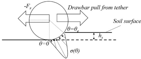
**Fig. 5.** Distribution of the normal stress under wheels on soil surface.
