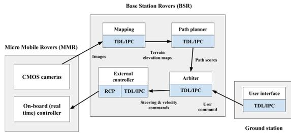
Fig. 6. Each component in an MMR’s navigation system communicates via message passing protocols listed below its block.
